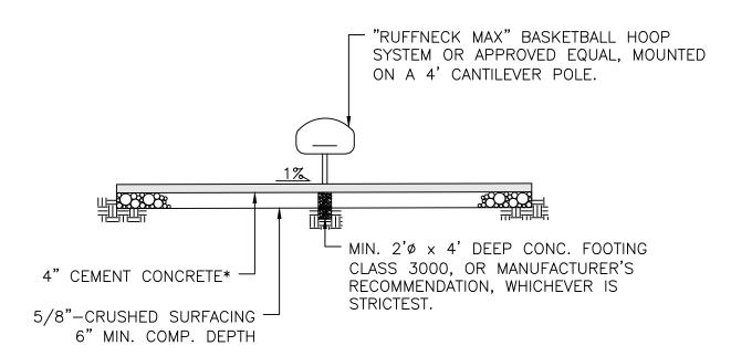
\*CLASS 3000 CONCRETE WITH TYPE III FIBER REINFORCEMENT, PER REQUIREMENTS OF ASTM C116. MIX DESIGN TO BE APPROVED BY CITY ENGINEER PRIOR TO PLACEMENT.
